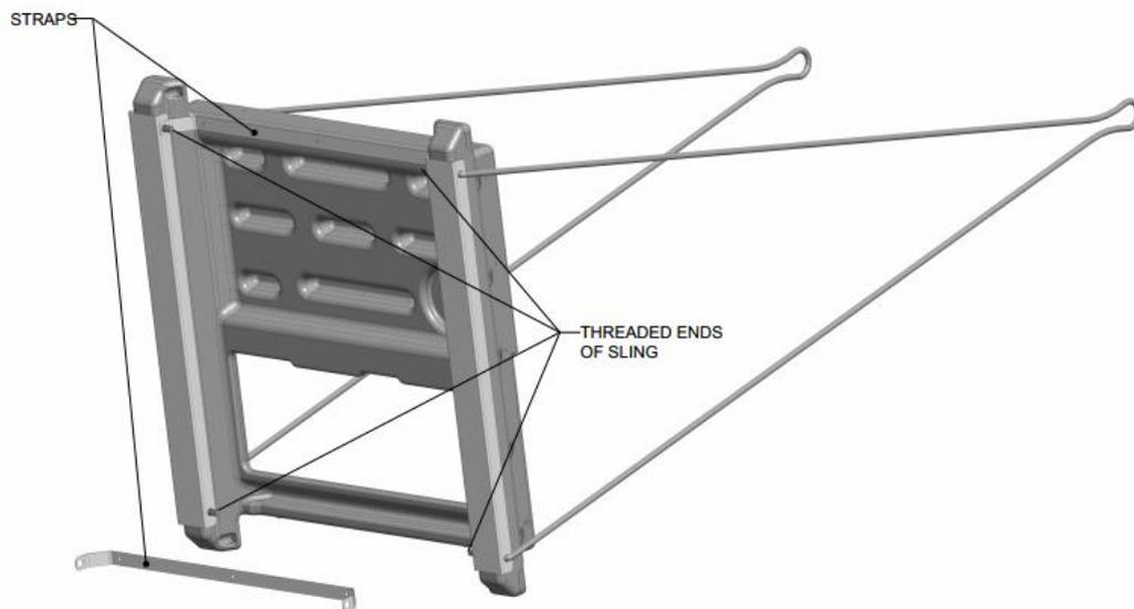
6. Install (in this order) on all (4) threaded ends of slings: 5/8" SAE washer, 5/8" lock washer, 5/8" slotted nut, cotter pin. Bend ends of cotter pin, after installed through hole in sling and slot in nuts, to secure.
