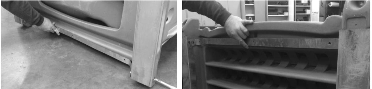
3. Transfer drill (4) 11/16" holes through the base using the holes in the cradles, **keep cradle flat against bottom of base skids.**
