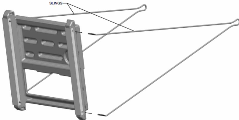
5. Install (2) straps along crossmembers and onto the threaded ends of the slings as shown.
